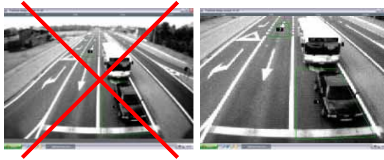
Figure 2: Bad and good camera image (illustration with wide angle TrafiCam)
